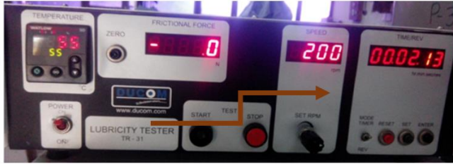
(c) Digital control device
